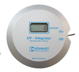
While on the conveyer belt, the UV-Integrator 150 can withstand max. 110° Centigrade for up to 10 seconds. The temperature of the housing should not exceed 45° Centigrade.
